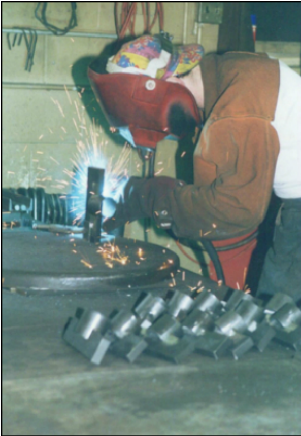
Welding rapper sockets
