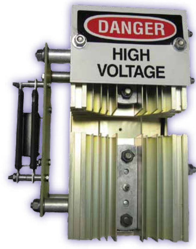
SILICONE CONTROLLED RECTIFIER (SCR)
